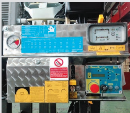
Comandi accessibili da terra. Tutti i carter in acciaio inox AISI 304. Controls can be reached standing on the side. All the carter are in stainless steel AISI 304. Commandes accessibles de terre. Tous les carter sont en acier inox AISI 304. Von der Seite steuerbar. schutzplatten in Edelstahl AISI 304.
